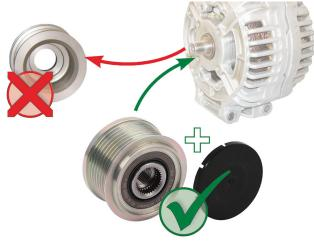
Changing from a rigid belt pulley to an Over-Running Alternator pulley
